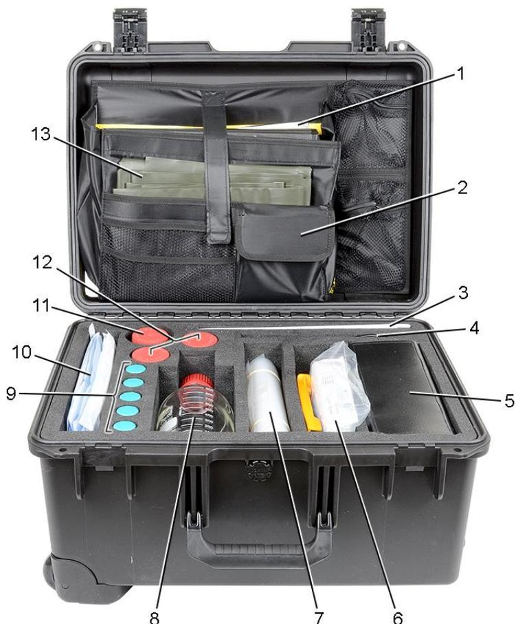
The sampling equipment is stored in a waterproof and shock absorbing plastic case.
