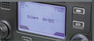
The transmit functionality of the A100 can be switched on and off whilst continuing to receive all AIS messages.
